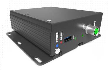
PS-ECU is a compact on-board computer for buses and trains, specially designed for video processing with AL. This edge computing unit combines high performance and compactness.
